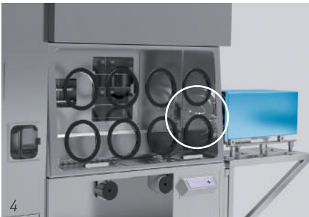
Close: at the end of the procedure, the RTP is closed allowing disconnection.
