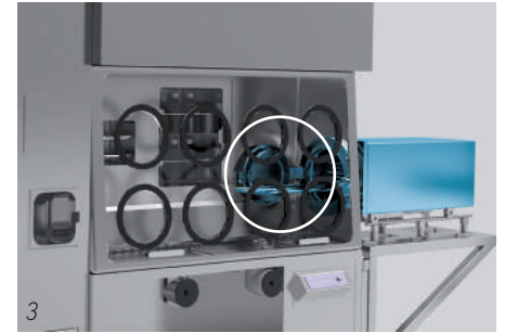
Connect and use: the incubator is aseptically connected by an RTP to the isolator and opened in a grade A environment.
