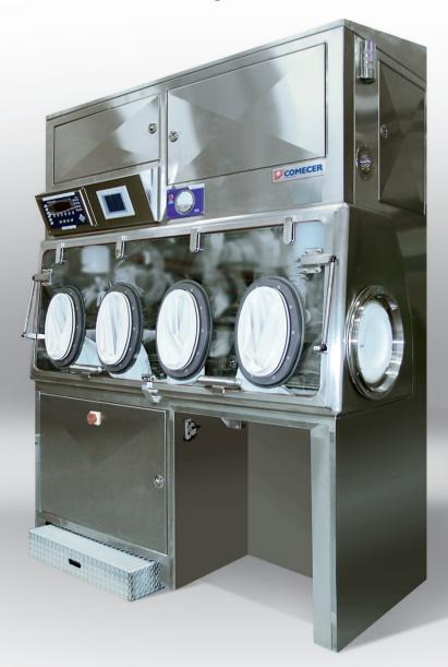
The isolator is designed to carry out weighing and powder transfer procedures (API) in complete safety. The isolator consists of a chamber equipped with connections for scales and cable runs, with a front wall in glass which can be opened completely.
