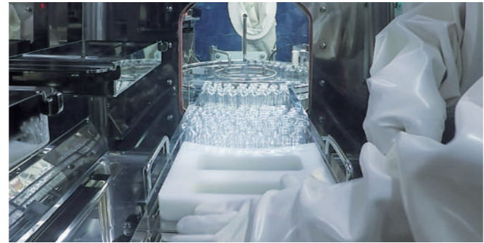
Empty vials are introduced manually into filling station through a loading chamber.
