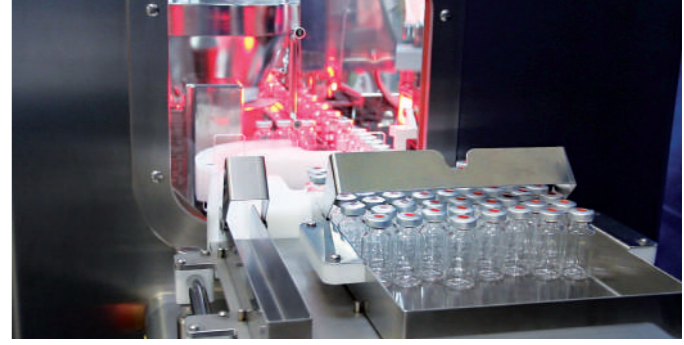
The filled/stoppered/crimped vials are automatically loaded on a specific tray.
